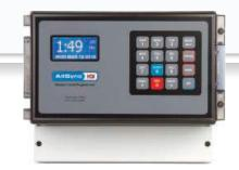
Some masters are equipped to synchronize their time to NIST via GPS or Ethernet for very accurate time.
