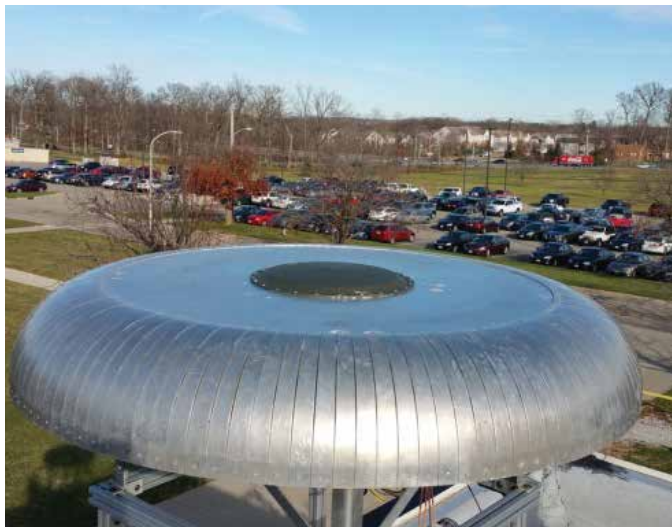
FIGURE 7 GAS-1 CRPA with 51-inch-diameter rolled-edge ground plane installed on the roof of the ANT Center.
