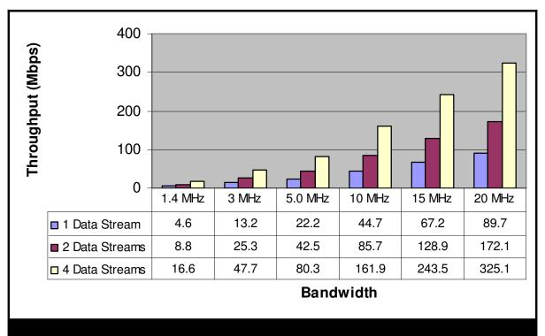
Figure 5 - Peak LTE Downlink Throughput with Single and Multiple Data Streams
