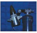
XM 982 Nosecone with Dualband L1-L2 GPS Antenna Array
