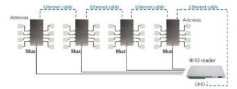
AdvanMux-8 can be controlled both by standard +5 V and open collector digital outputs.
