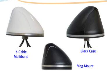
The SMW-311 Series antennas features 3 antenna elements in one radome. The unique feature of this model is that the cellular element (Cable 1) is extremely widebanded and can cover the traditional GSM/CDMA frequencies, 700 MHz LTE, 1.7 & 2.1 GHz AWS/UMTS bands and LTE/WiMAX at 2.5 or 3.7 GHz, all on a single board.
